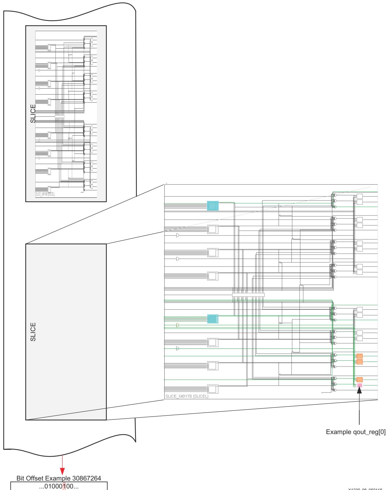
Figure 8: Example Readback Capture Representation of CLB Register from Reference Design
