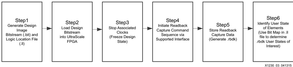
**Figure 3: Readback Capture Flow Overview**
