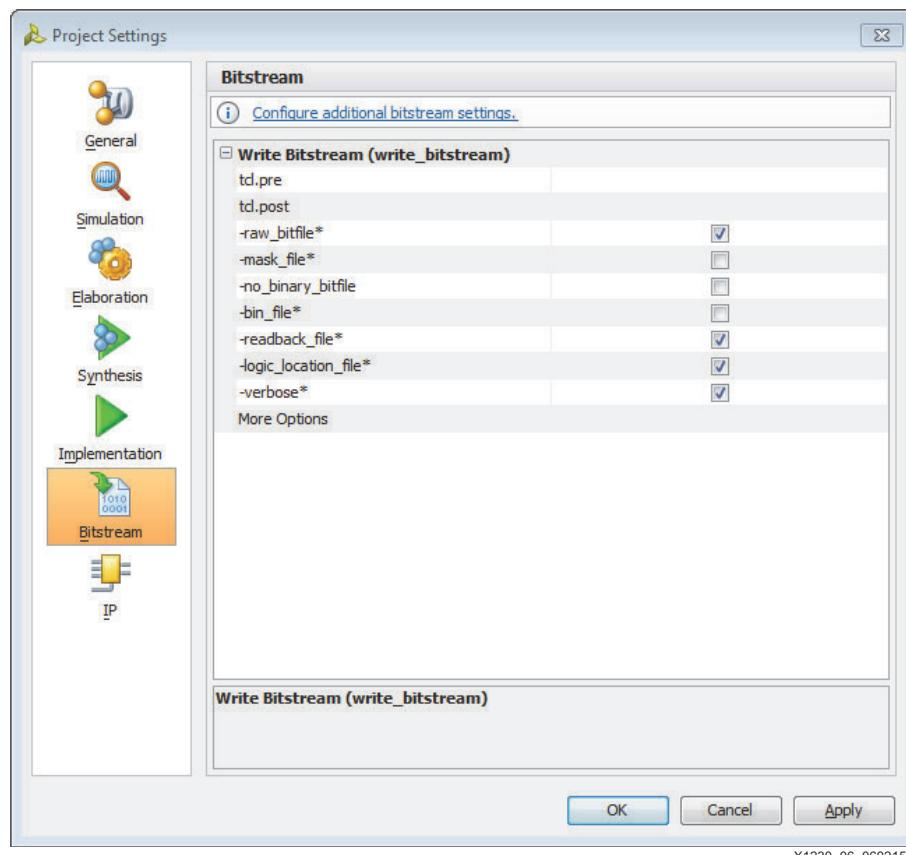
Figure 6: Vivado Design Suite IDE Bitstream Settings
