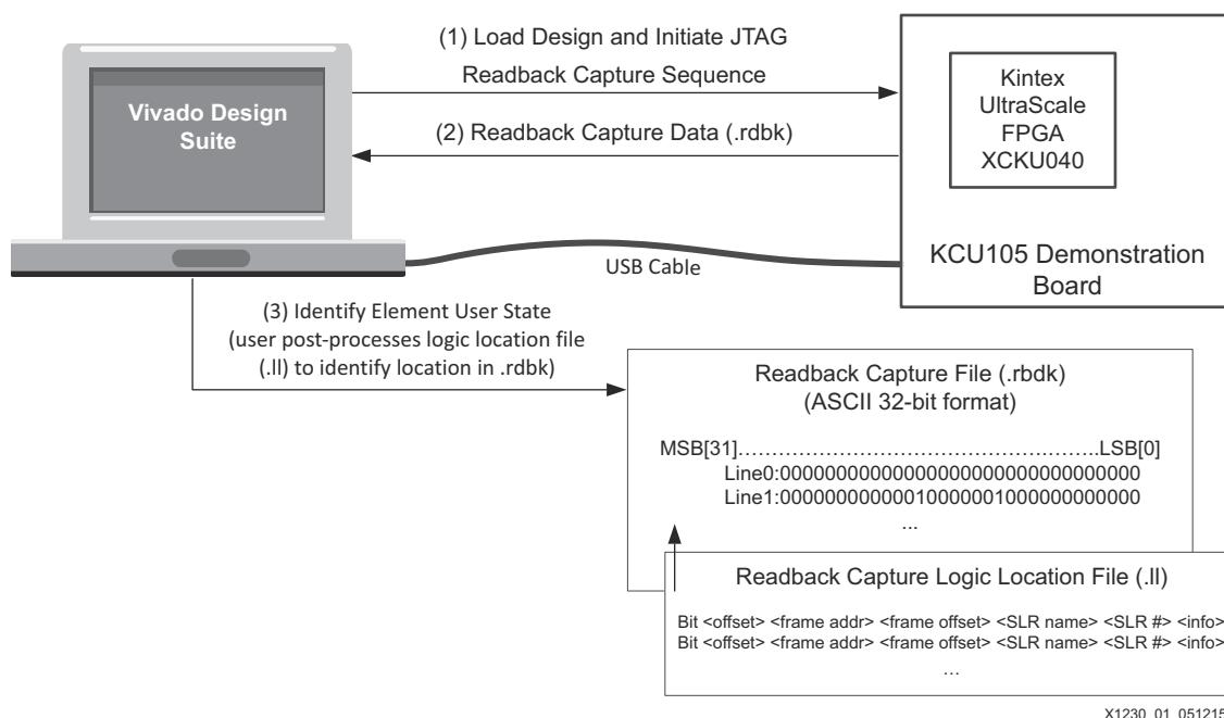
Figure 1: UltraScale FPGA Readback Capture Flow via JTAG Interface
