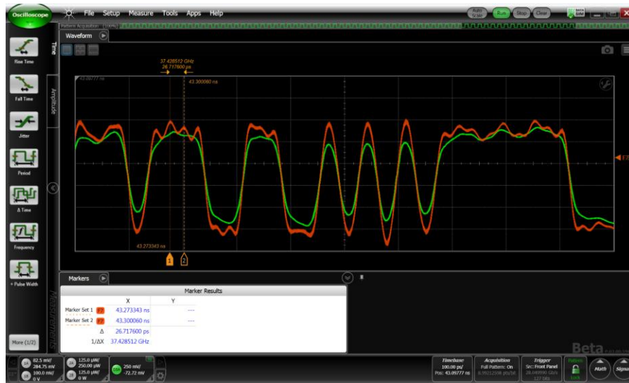
Figure 24: Ringing on a de-embedded signal (F7 Orange in this case) is often caused by S-parameters with excessive loss, or insufficient bandwidth.
