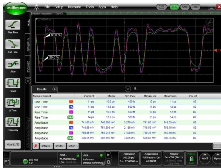
Figure 23: Comparison of three de-embedded signals (F3 Pink, F5 Blue, and F7 Orange) with the raw input signal (D1A Green) using a PRBS15 pattern.
