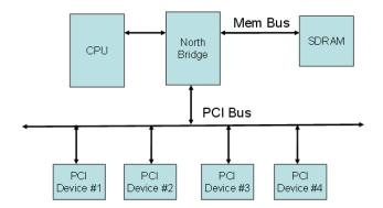
In this example, let's assume the device generating the interrupt is device #3. Let's also assume that Device #1 and Device #3 share the same IRQ.
